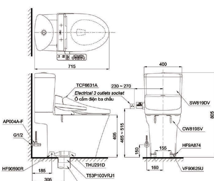
⊕: Electrical 3 outlets socket (must have really ground connection phase), type G.
